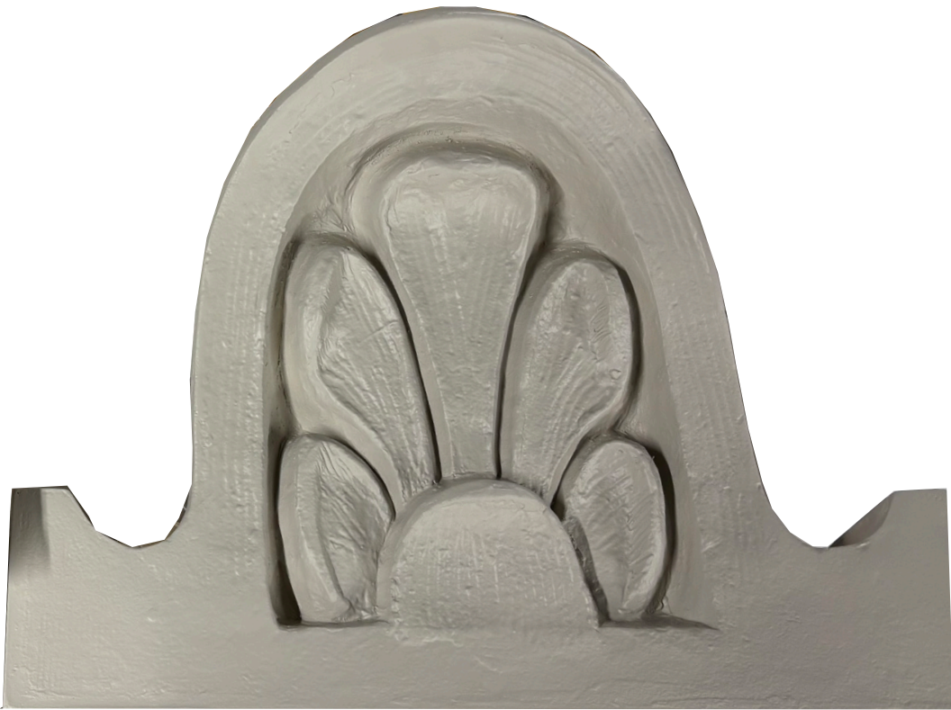
Uncoated GFRP sample Coating color & sheen to be colormatched
