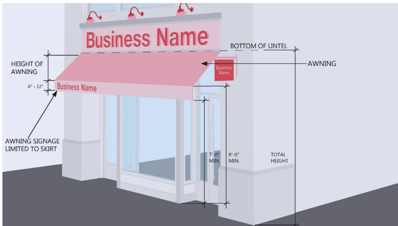
Typical storefront awning location and dimensions.
