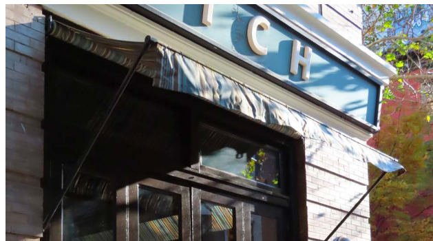
A retractable storefront awning installed at the top of the storefront infill within the opening.
