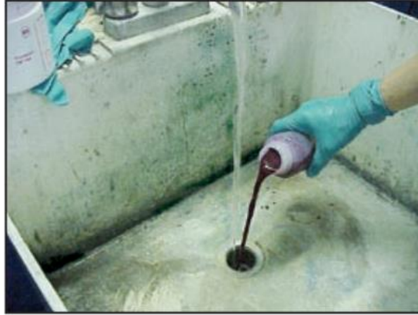
Image 46. Dye testing – introduction of dye (source: EPA Guidance Manual p. 160)
