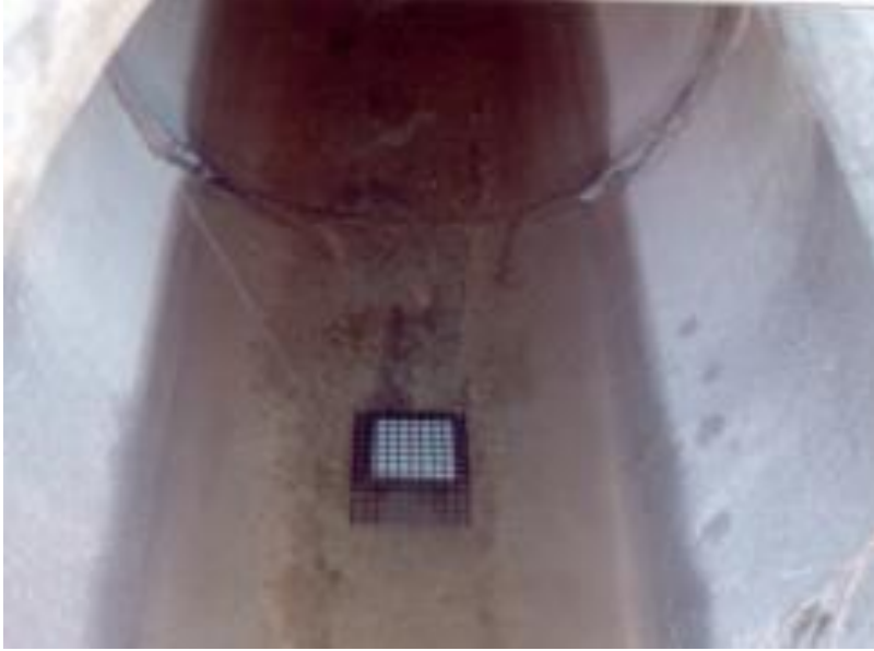
Image 53. Optical brightener monitoring device deployed in a storm sewer (source: Galveston County (TX) IDDE Manual, 2002)
