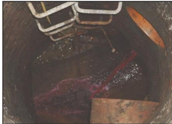
Image 7. Dye testing – observing dye downstream (source: EPA Guidance Manual p. 161)
